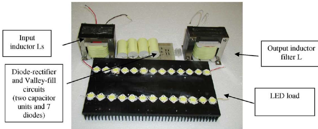
Figure 7: Components of the demonstrator circuit of the passive LED driver for street lighting [18].
