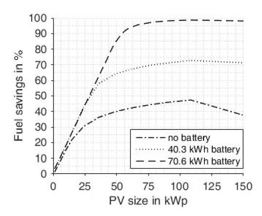
57 kWp PV and 70.6 kWh battery save aprox. 81 tons of CO<sub>2</sub> in 20 years (life time period)
