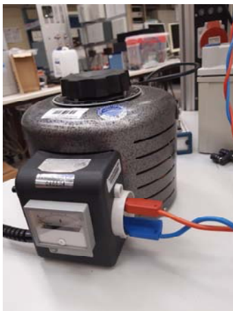
Figure 13: Transformer for voltage control
